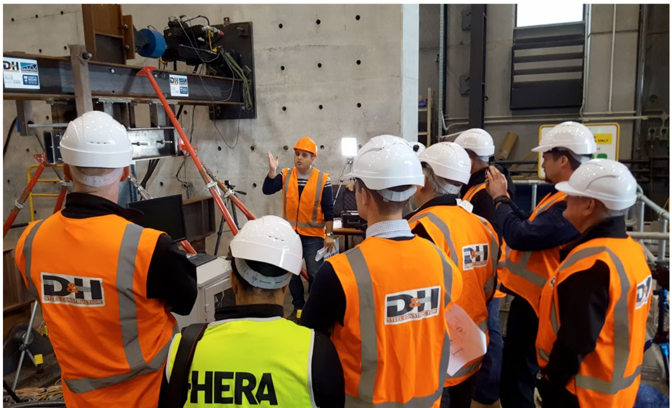
Impact and Value of HERA's Research and Training of Researchers -Low cycle fatigue test of a large scale welded moment resisting connection at the University of Auckland
