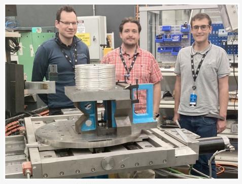
Residual Stress Measurement of Additive Friction Stir Deposition on aluminium components on the Kowari Strain Scanner at ANSTO – Research team, University of Sydney
