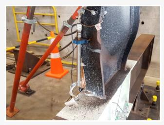
HERA Seismic Research Programme, low cycle fatigue testing of a welded moment resisting frame connection at the University of Auckland, New Zealand [104]
