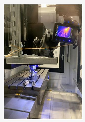
Additive Friction Stir Deposition experimental set-up at Advanced Manufacturing Research Centre (AMRC)
