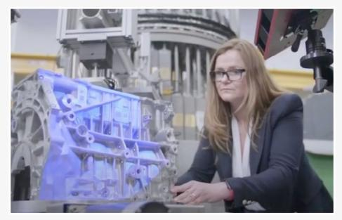
Setting-up an aluminium engine block for residual strain measurement
