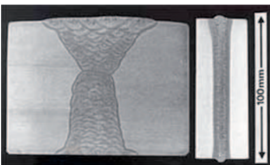
Figure 5.3 Comparison of single pass EB weld profile with multi pass submerged arc welded joint in 100 mm thickness C-Mn steel (Reproduced courtesy: B. Pekkari)
