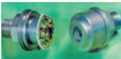
Pressure sensor incorporating, laser, electron beam and thermosonic welding
