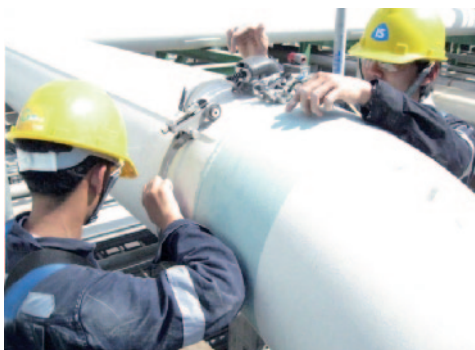
Figure 5.15 Phased array inspection in lieu of radiographic inspection on welds in piping (according to ASME B31.3) (Reproduced courtesy: Institut de Soudure)
