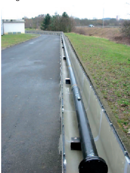
Figure 5.19 Testing loop built to assess performance of guided waves (Reproduced courtesy: Institut de Soudure)
