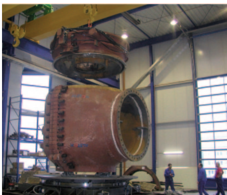
Figure 4.8 Housing of a gas turbine being prepared for EB welding (Reproduced courtesy: Probeam)
