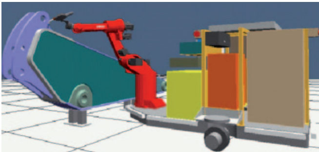
Figure 5.2 Robot with all its equipment mounted on a RTV welding a large structure (Reproduced courtesy: TWI Ltd)
